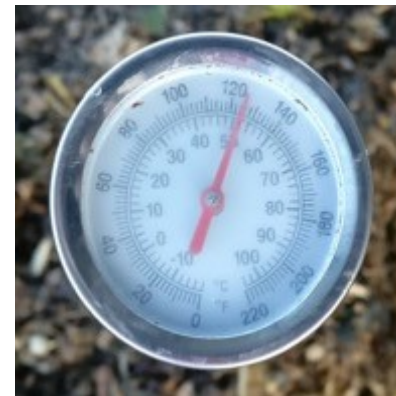
Thermal control : 1 st week 70°C second week 40°-50°C , and third week temperature was stable at 40°C.
